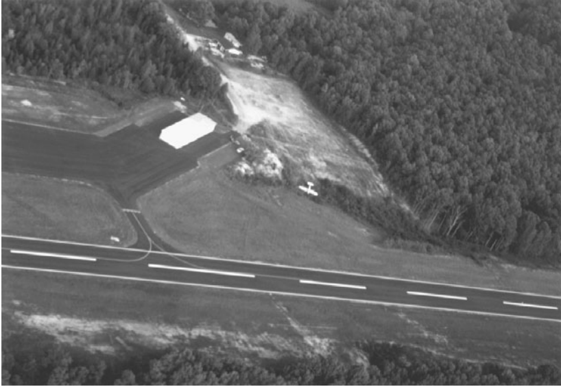
Figure 6.2D The airplane had been landing from left to right. The taxiway intersection where the airplane left the runway and the airplane itself can be seen in this aerial view of the accident.
