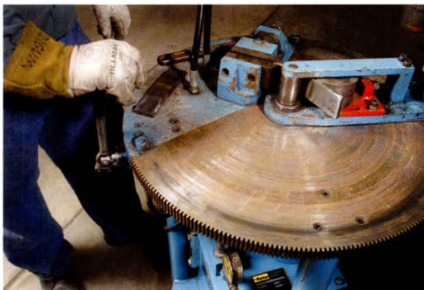
The sample strip is clamped in a motorized wrap-around-bend test jig. Monte Swann
