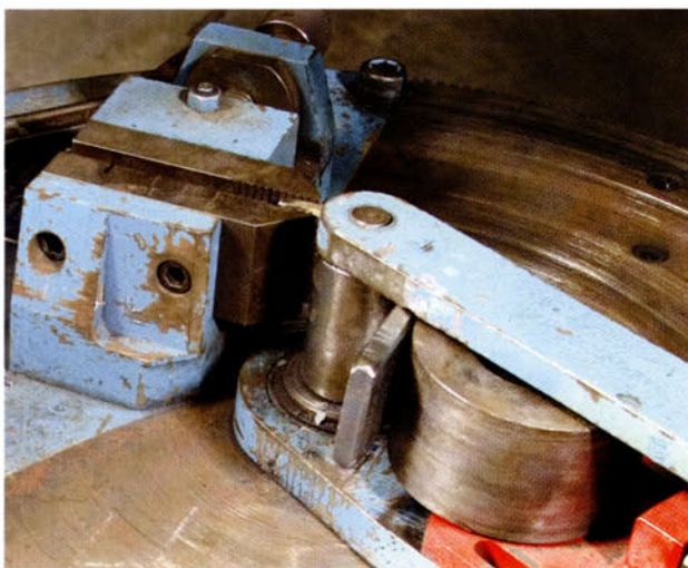
The test strip is wrapped around a 1½-inch diameter mandrel. Monte Swann
