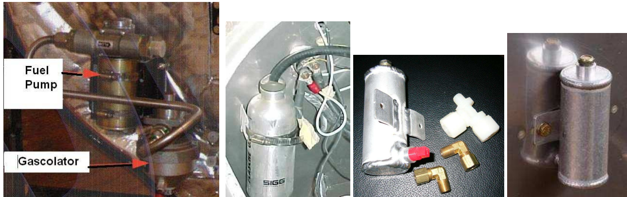
Picture 7 Fuel Pump and Gascolator (left), Coolant Overflow Bottle (center), Brake Fluid Reservoirs (right)
