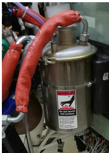
Picture 8 Remote Oil Reservoir and Attachment Bracket, Rotax
