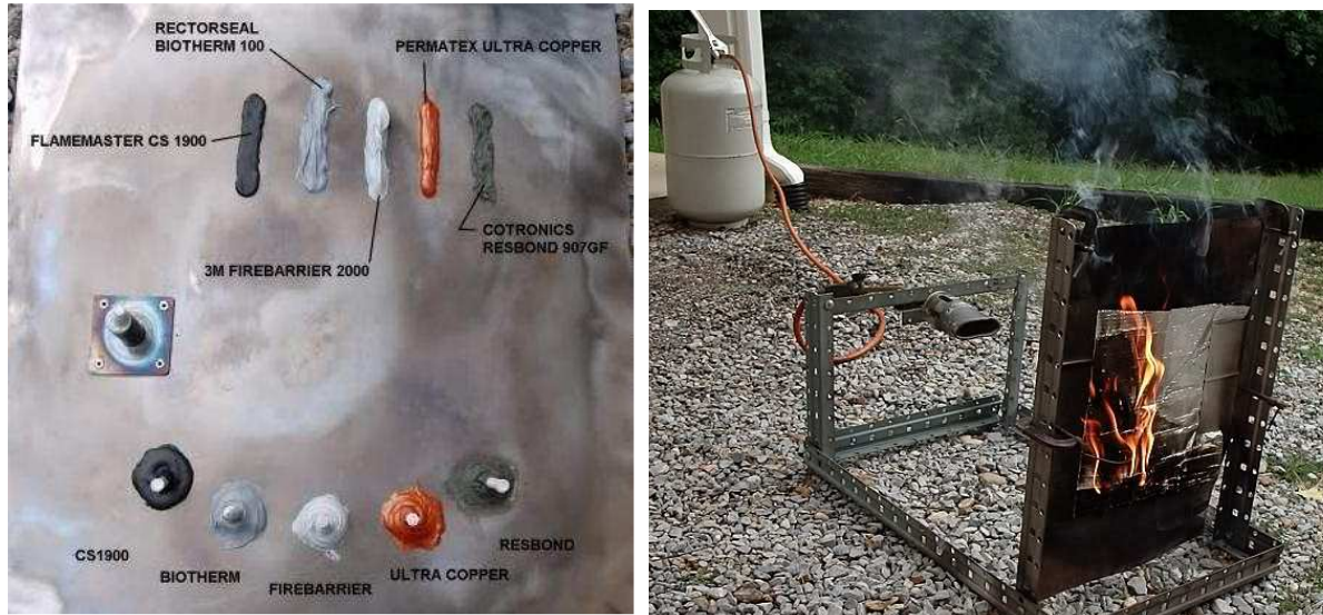
Picture 5 Sealant Burn Test Setup
