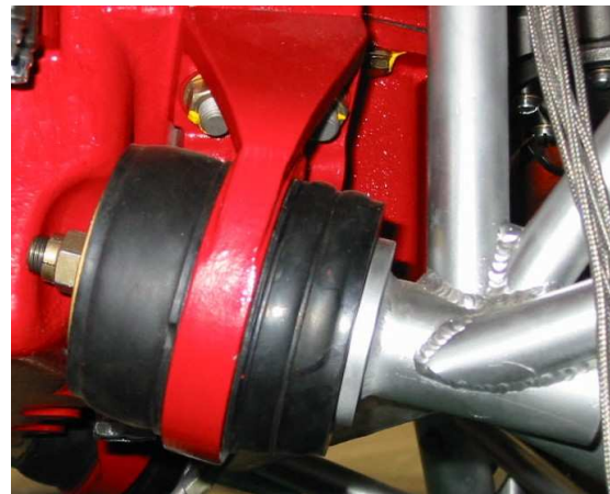
Picture 11 Dynafocal Shock Mount Assembly, Continental Style (left), Lycoming Style (right)
