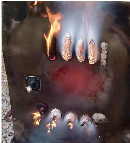
Picture 5 Sealant Burn Test Setup
