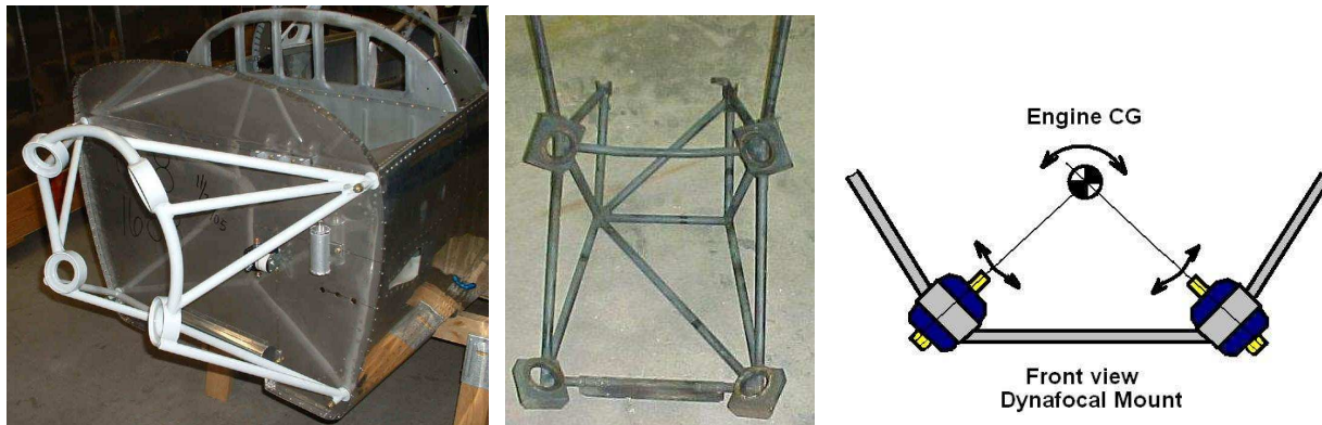
Picture 9 Rear Engine Mount for Lycoming Engine (left), Bedmount Style (right), Concept Dynafocal Mount
