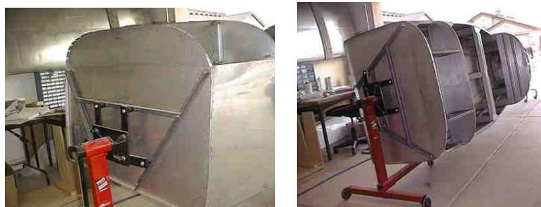
Another possibility is buying an engine stand and fabricating some 1/4 inch steel angle to fit the engine mounting holes on the firewall. This stand allows you to move the fuselage around the shop and you can rotate it when working inside or on the bottom of the fuselage.
