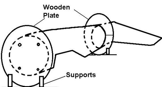
A very simple jig consists of round pieces of plywood. The fuselage can be rolled around on the floor to any angle only limited by the vertical tail. It is low enough to easily work on. The height is
