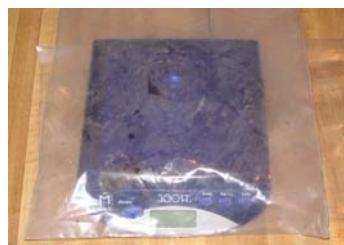
An electronic scale is the most useful tool for measuring resin in the correct proportions. Unfortunately it seems to be impossible to pour resin into a cup on the scale without spilling some. I put the scale in a plastic bag to protect it. I can push the buttons and read the display through it. When it becomes too sticky, I replace the bag.
