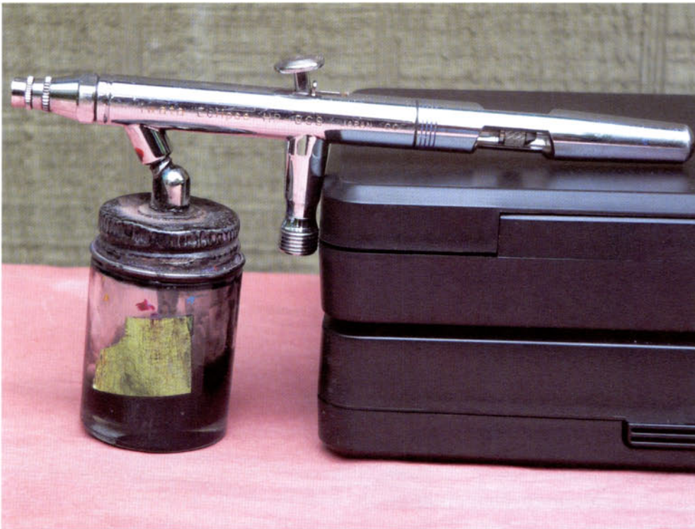
This is a siphon-feed airbrush, also known as a bottom- or bottle-feed. T-shirt airbrushers tend to prefer this airbrush because they use a wide variety of colors at once, and the bottle-feed makes it possible to quickly and easily change colors using one airbrush. Pictured is an Iwata Eclipse HP-BS.
