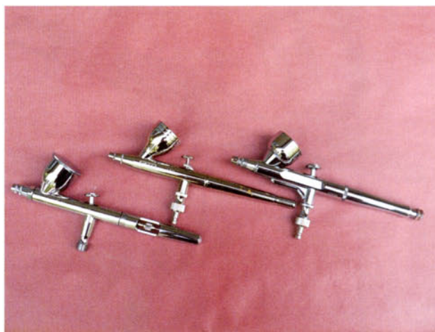
Above left: The Richpen 013G, a single-action, internal-mix airbrush. Above right: A few different brands of dual-action airbrushes that I use and recommend, from left to right: Iwata Eclipse, SATAgraph 3, and Richpen 213C.
