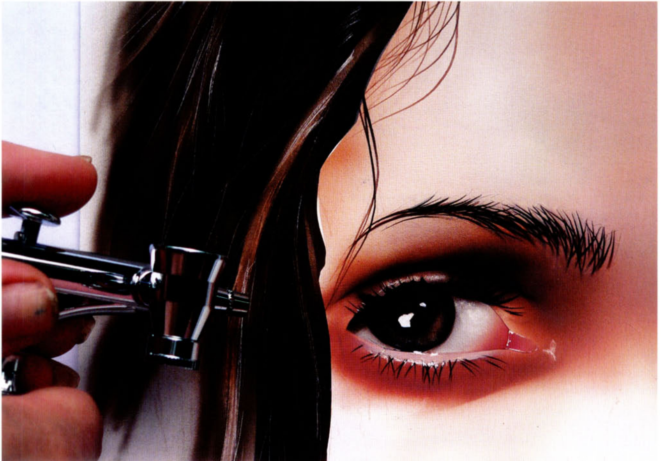
An external-mix airbrush, the Paasche HS#1 single-action.
