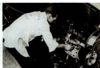
• 274-inch Merc used Harmon and Collins mags, Sharp heads and manifold. Art Chrisman worked hands over to handle mixtures of 75% nitro, 25% alcohol. Speed record was in carterhouse.
