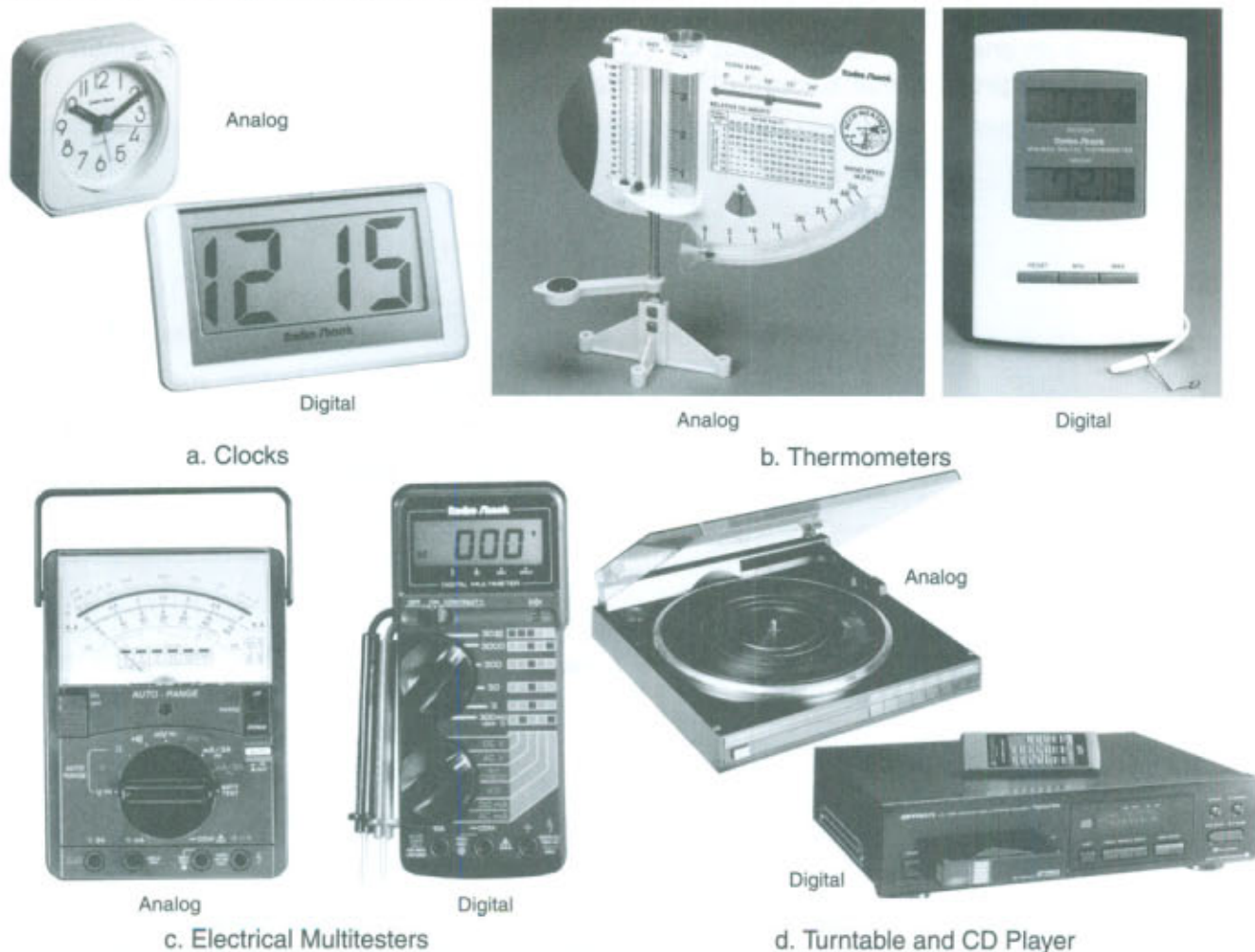
Figure 1-3. Examples of the same quantities (time, temperature, electrical values, and sound) represented both as analog and digital values.
