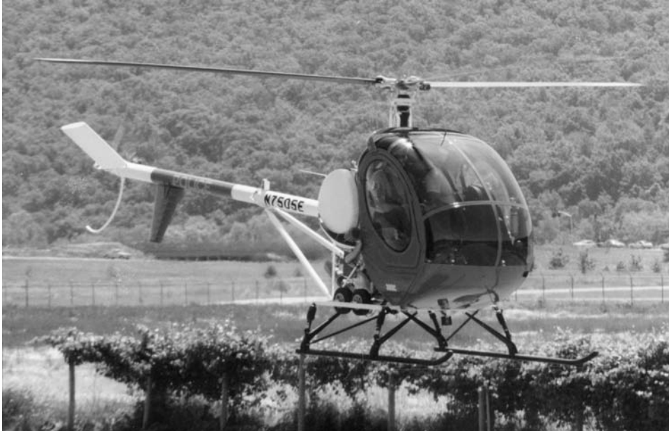
FIGURE 1-4 At the hands of a skilled pilot, a helicopter can make an engine-out landing into an area not much larger than the helicopter itself: Schweizer 300. (Source: Schweizer Aircraft Corporation)
