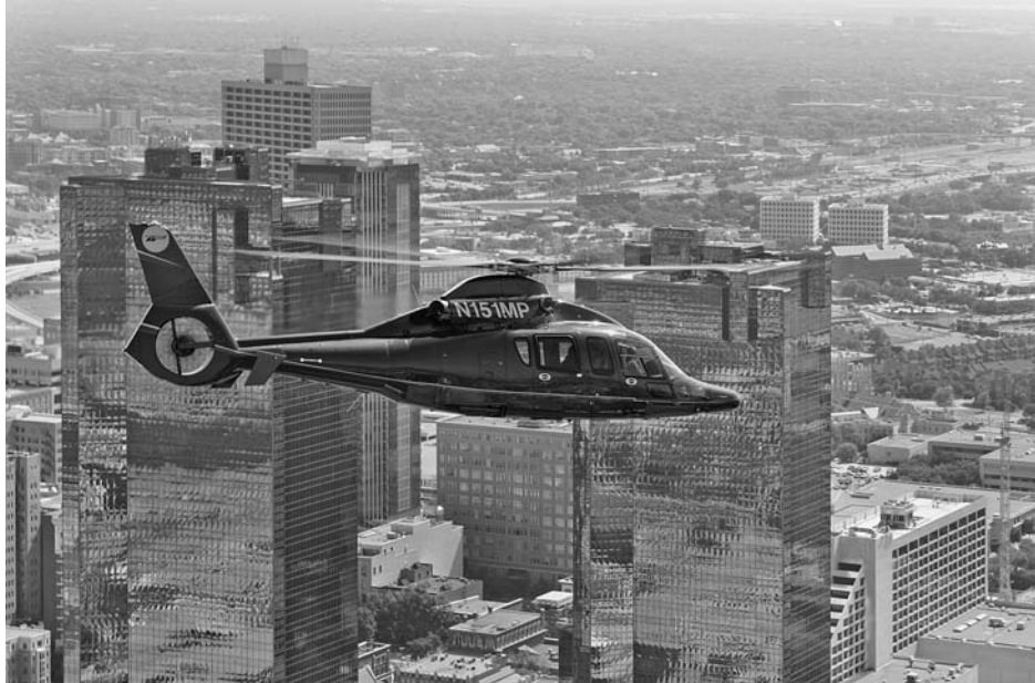
FIGURE 1-6 If one engine fails in a twin-engine helicopter, the flight can be continued to the nearest safe landing area: Eurocopter EC155. (Source: Eurocopter)
