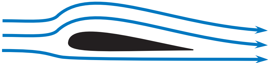
FIGURE 1.2 Based on Newton's laws, this wing has no lift.
