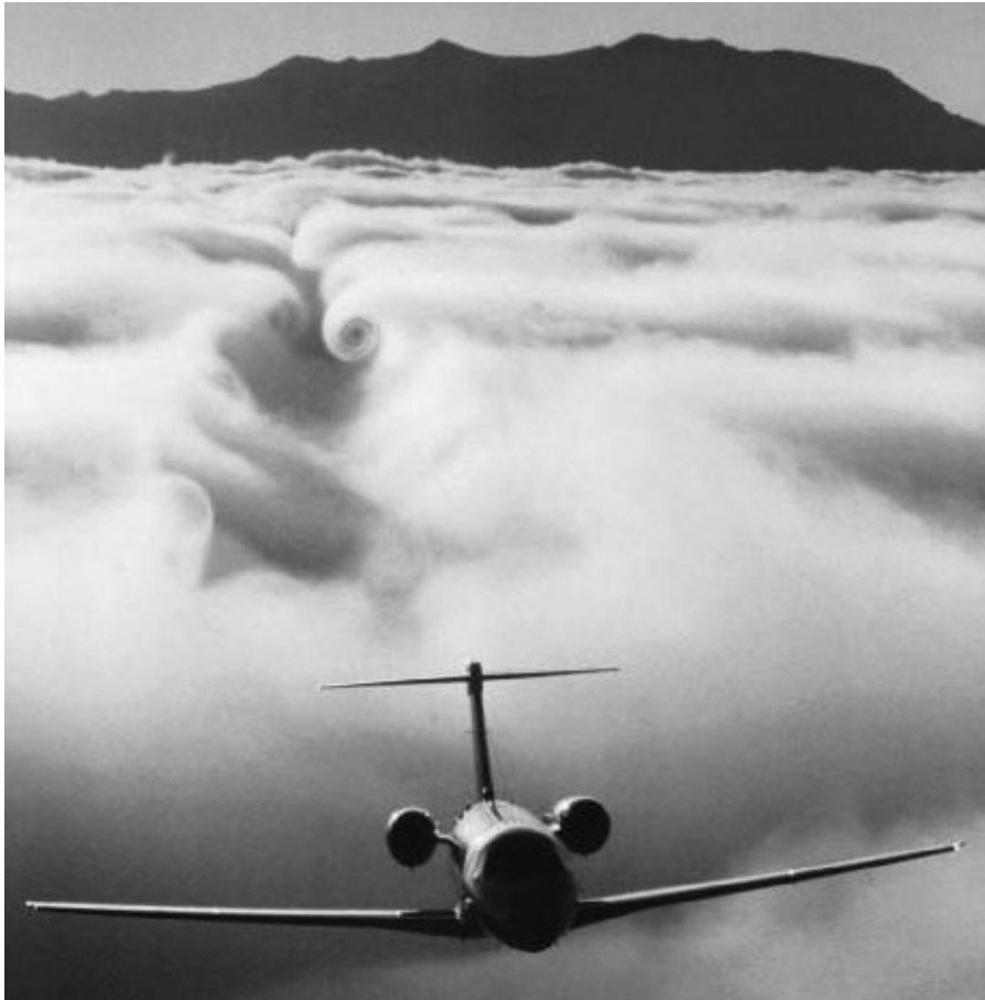
FIGURE 1.7 A jet flying over fog demonstrates downwash. (Photograph by Paul Bowen; courtesy of Cessna Aircraft Co.)
