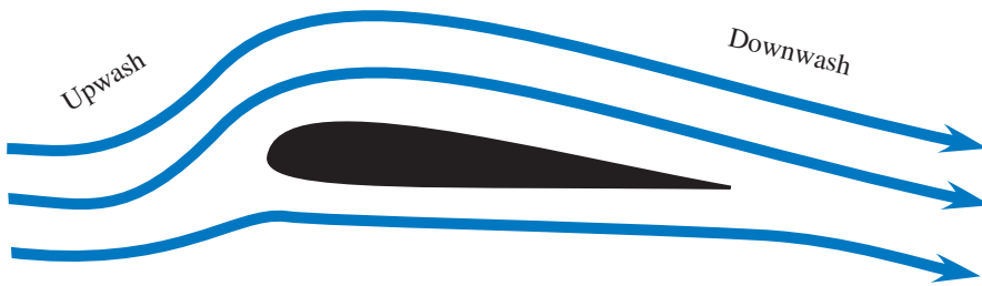
FIGURE 1.3 The airflow around a real wing with lift.
