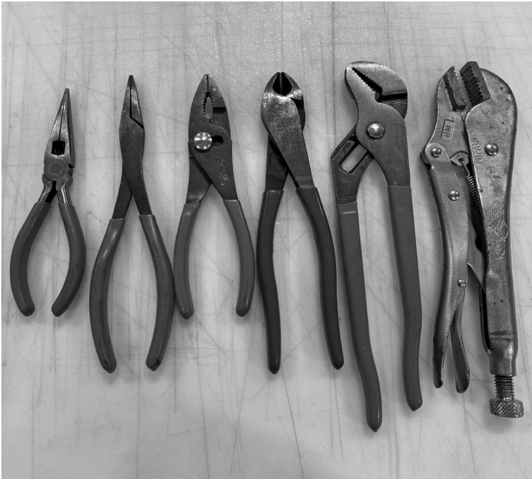
FIGURE 2-3 Types of pliers (from left to right: needle-nose, duckbill, diagonal cutter, and water-pump pliers).
