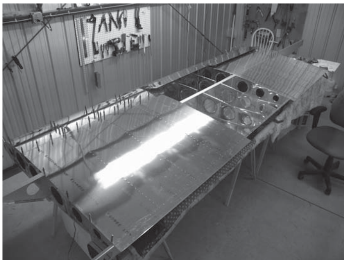
Figure 1-1 Photo of the Van's RV 12 LSA experimental aircraft wing displays the main and rear spars (solid, lengthwise rails)—and attached ribs, which give the wing its shape and added strength. (Photo courtesy of Jim Olson, NC.)
