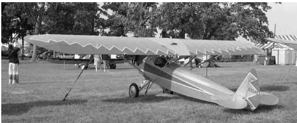
Fig. 1-4. The Heath Parasol was the first mass-marketed kitplane. This is a Super Parasol, slightly larger and more powerful than the original.
