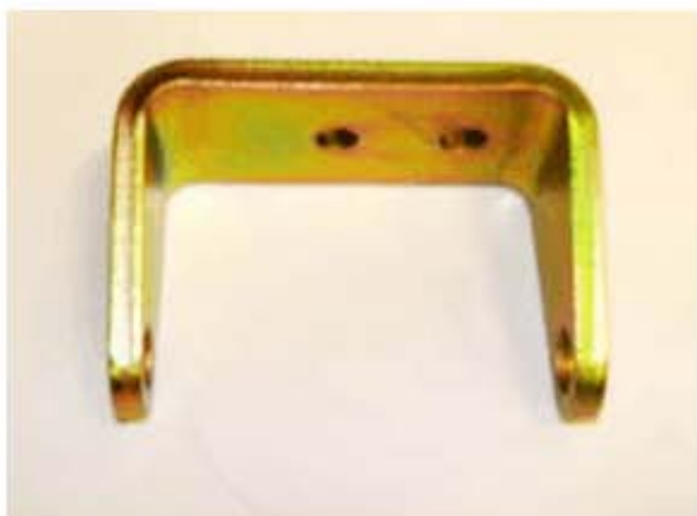
Figure 3-7. Exemplar Lycoming Boss-Mount Alternator Bracket - BEEFY!
