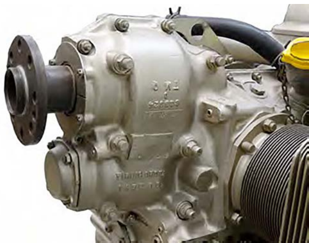
Figure 3-31. Spur-Type propeller gear reduction system.
