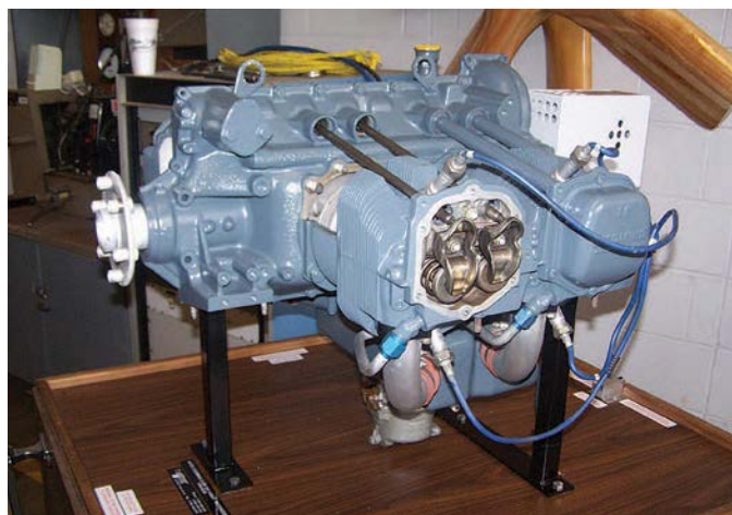
Figure 1-8. Four-cylinder opposed engine.
