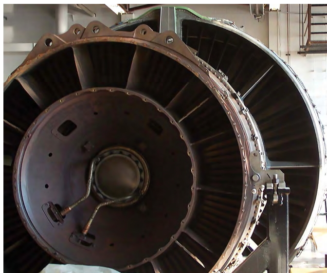
Figure 3-8. Air from the fan exhaust can be discharged overboard through short ducts directly behind the fan.
