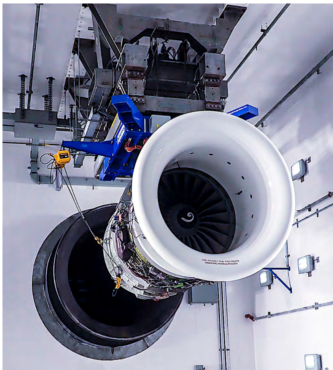
Figure 3-15. Bellmouth inlet mounted on test cell engine.
