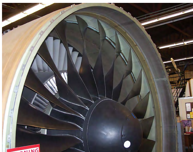
Figure 3-7. The air that passes through the inner part of the fan blades becomes the primary airstream.
