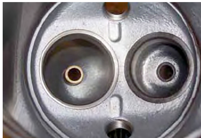
Figure 1-18. View of cylinder head showing valve seats, valve guides, and spark plug holes.
