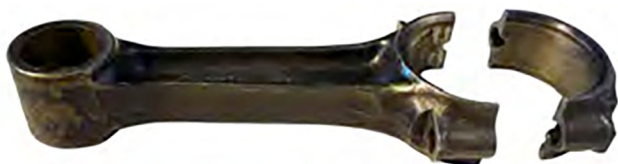
Figure 1-16. Plain-type connecting rod and cap assembly.
