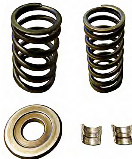
Figure 1-21. Inner and outer valve springs, valve spring cap, and valve stem keepers.
