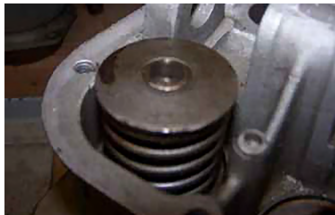
Figure 1-19. Valve installation showing valve tip, valve springs, valve spring cap, and valve stem keepers.
