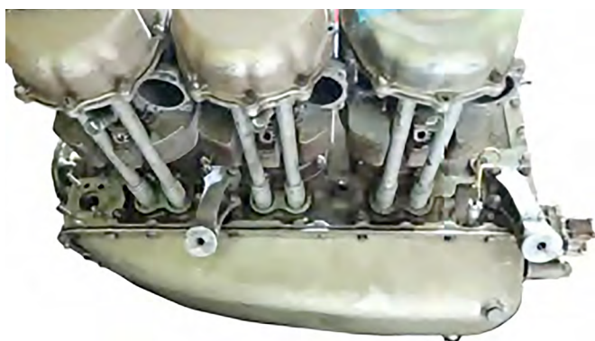
Figure 1-13. Wet sump engine.
