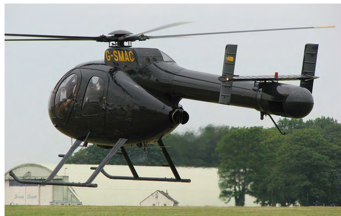
Figure 2-29. MD-520 helicopter with no tail rotor.
