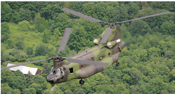
Figure 2-24. Tandem main rotor helicopter.
