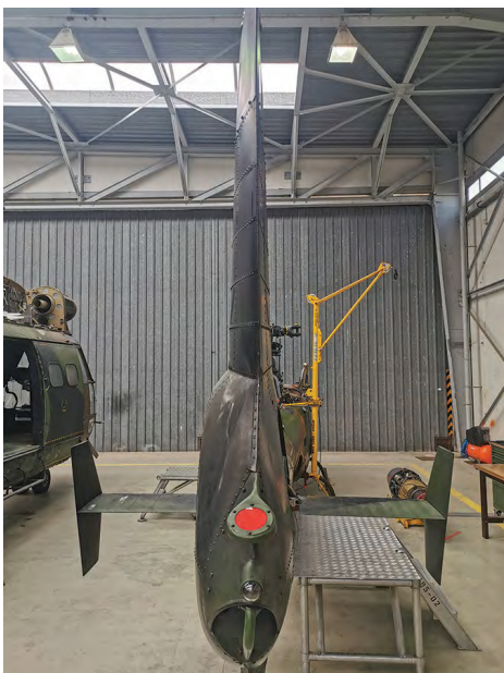
Figure 2-28. Fenestron dissymmetric vertical fin.
