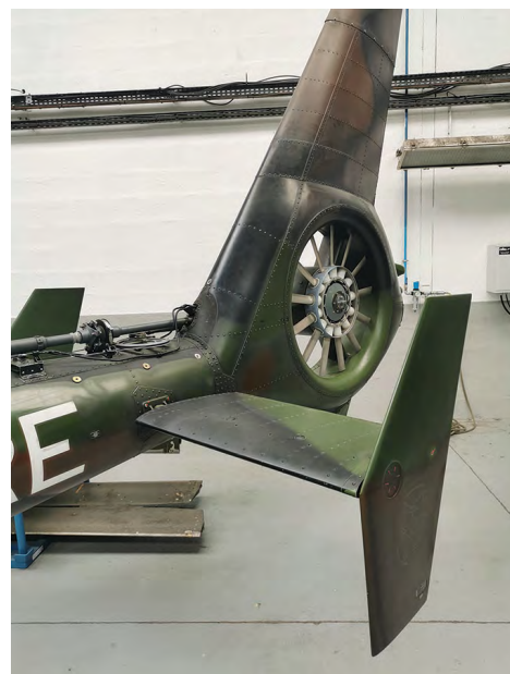
Figure 2-27. Fenestron on a Eurocopter Model SA341 Gazelle.
