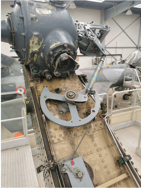
Figure 2-23. Cables-rear sector-rod and tail servo-control.
