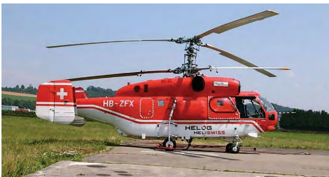
Figure 2-25. Helicopter with coaxial counter-rotating main rotors.
