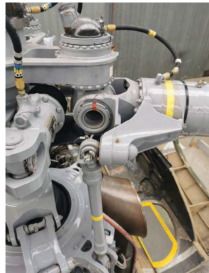
Figure 2-33. Fully Articulated Main Rotor System.
