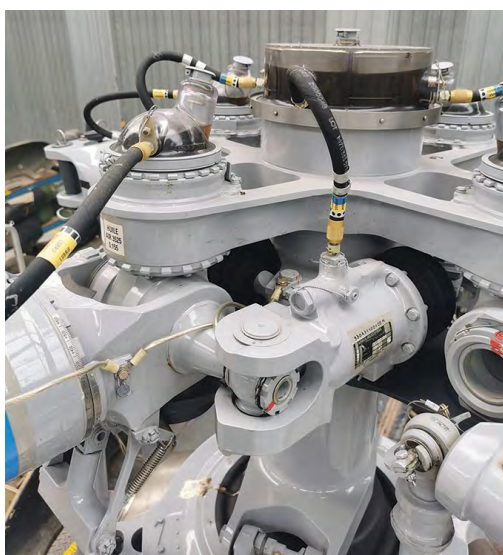
Figure 2-35. Drag hydraulic damper on SA330 puma.
