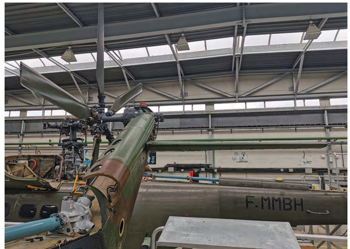
Figure 2-26. Aerospatiale Helicopter Tail Rotor.
