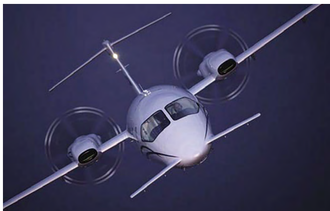
Figure 1-12. The Piaggio P180 includes a variable-sweep canard design, which provides longitudinal stability about the lateral axis.
