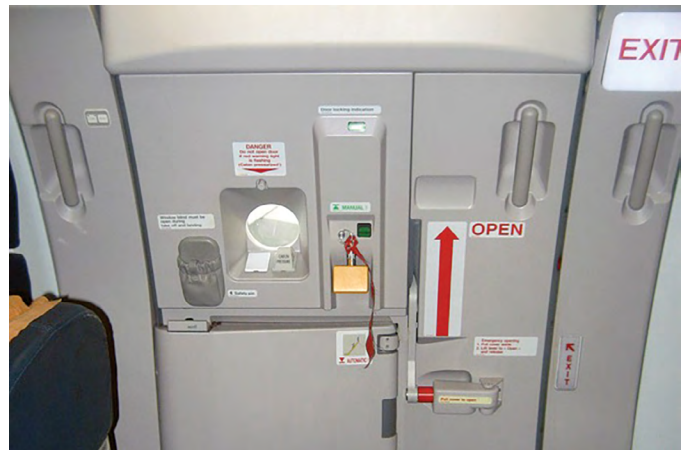
Figure 5-4. Required emergency exit markings.
