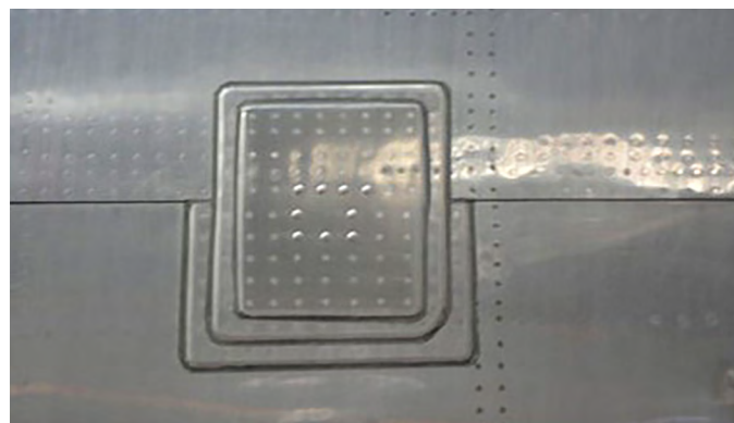
Figure 7-6. Photographic documentation of a repair is typical as a part of its work completion records.
