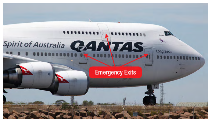
Figure 5-5. Required external emergency exit markings.
