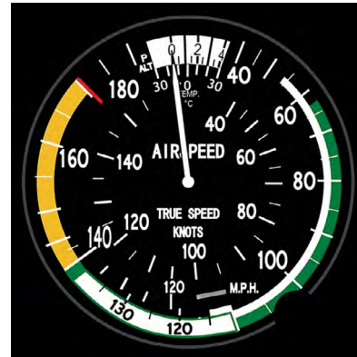
Figure 5-3. An airspeed indicator includes colored markings around its perimeter, highlighting important restrictions for which the pilot must be aware.
