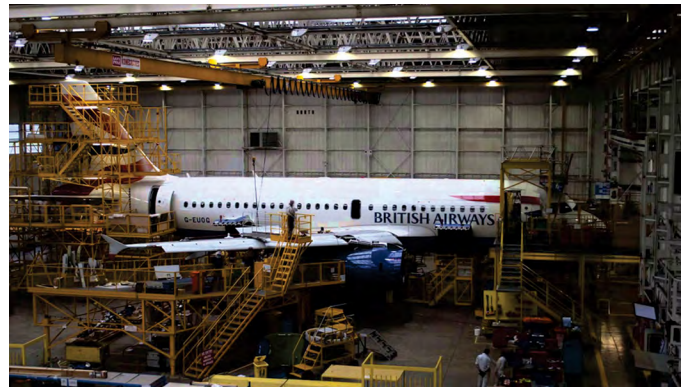
Figure 7-4. "C" Check inspection.
