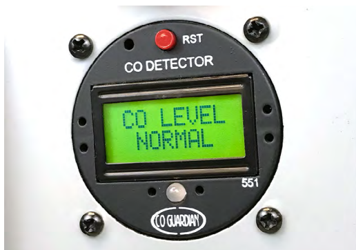
Figure 5-2. Many types of CO detectors will quickly warn of an emerging situation.
