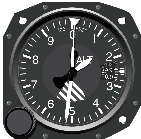
Figure 1-3. An airplane's altimeter is an aneroid barometer.
