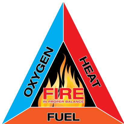
Figure 1-12. The fire triangle; all three elements shown are required for fire to occur.
