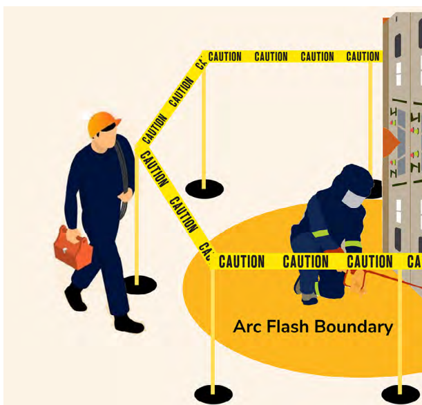
Figure 4-5. Setting up boundary areas when arc flash is possible will help reduce the risks of heat and arc blasts to unprotected personnel.
