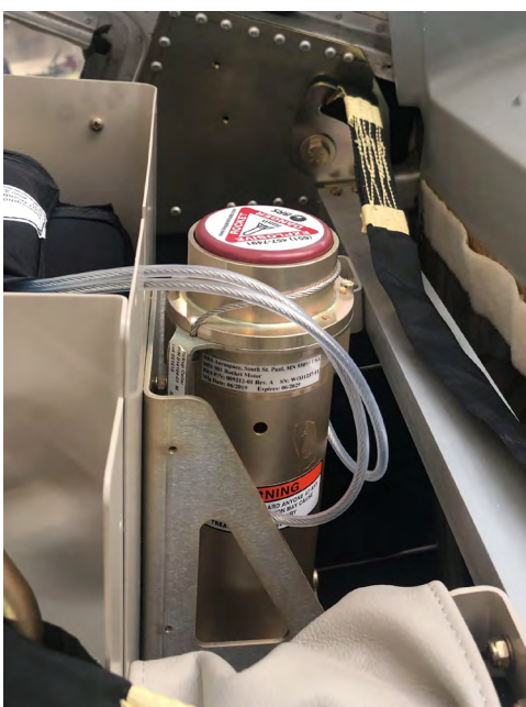
Figure 1-10. The internal mounting of a ballistic parachute system in a Cessna 182. Notice the rocket firing position through the rear window.
