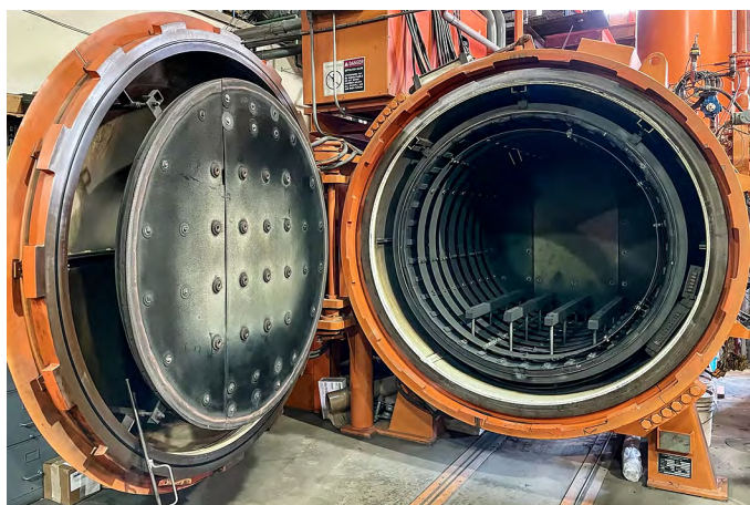
Figure 1-2. A heat treating furnace used to manufacture aircraft landing gear.
