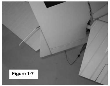
fixed trim tab is shown on the rudder in Figure 1-7.
