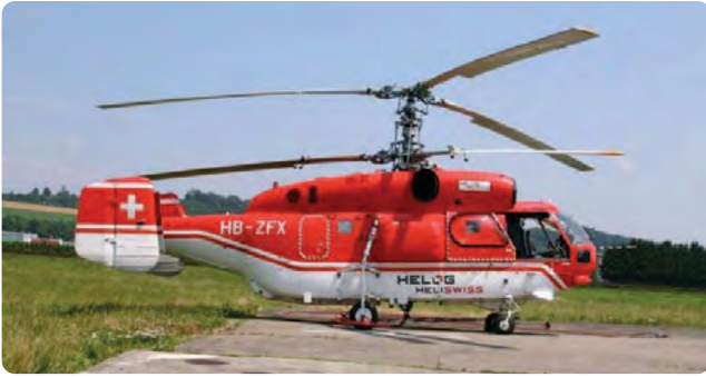
Figure 1-11. Coaxial main rotor helicopter.
