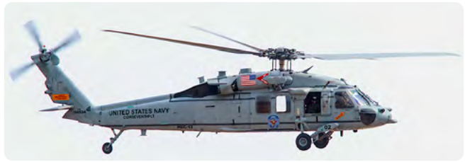
Figure 1-14. Tilt of main rotor during forward flight (Sikorsky H-60).
