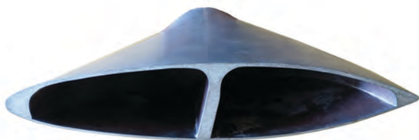
Figure 2-8. Cross section of steel propeller blade.
