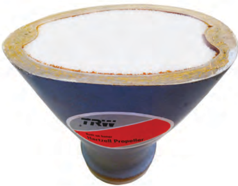
Figure 2-10. Cross section of composite propeller blade.
