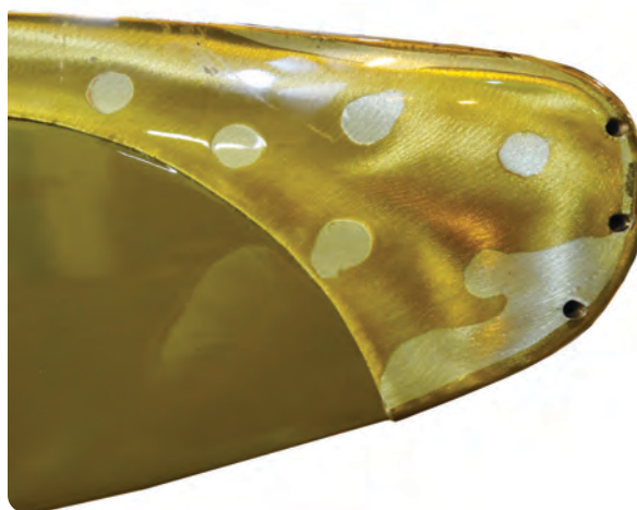
Figure 2-5. Tip on wooden propeller revealing soldered attachment hardware and drain holes.
