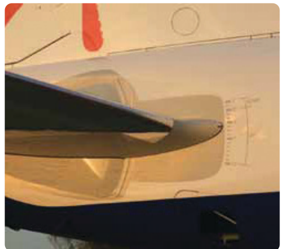
Figure 1-10. A stabilizer and index marks on a transport category aircraft.
