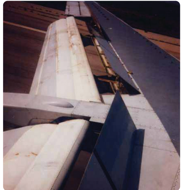
Figure 1-9. Spoilers deployed upon landing a transport category aircraft.
