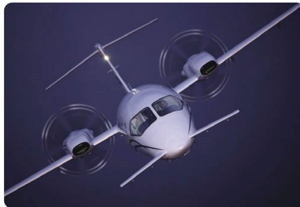
Figure 1-12. The Piaggio P180 includes a variable-sweep canard design, which provides longitudinal stability about the lateral axis.
