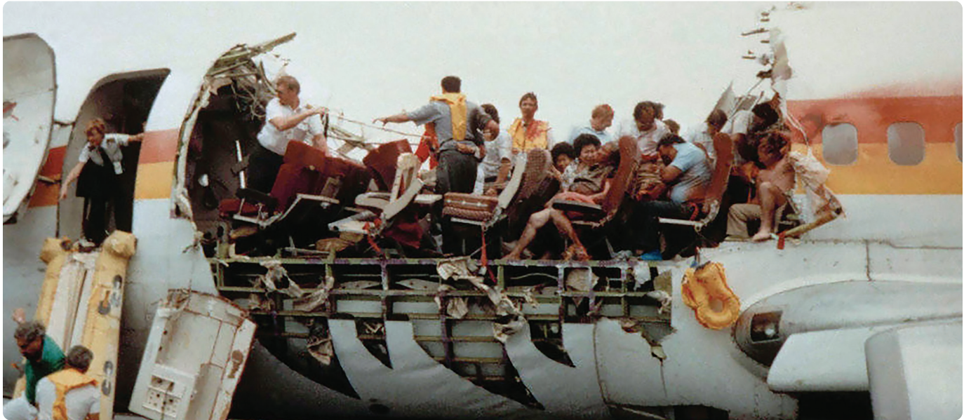
Figure 1-3. Aloha Airlines Flight 243; A watershed moment in aviation maintenance history that brought about much needed change in aviation maintenance. It was recognized that complacency in the state of aging aircraft was the main contributing factor to this accident.
