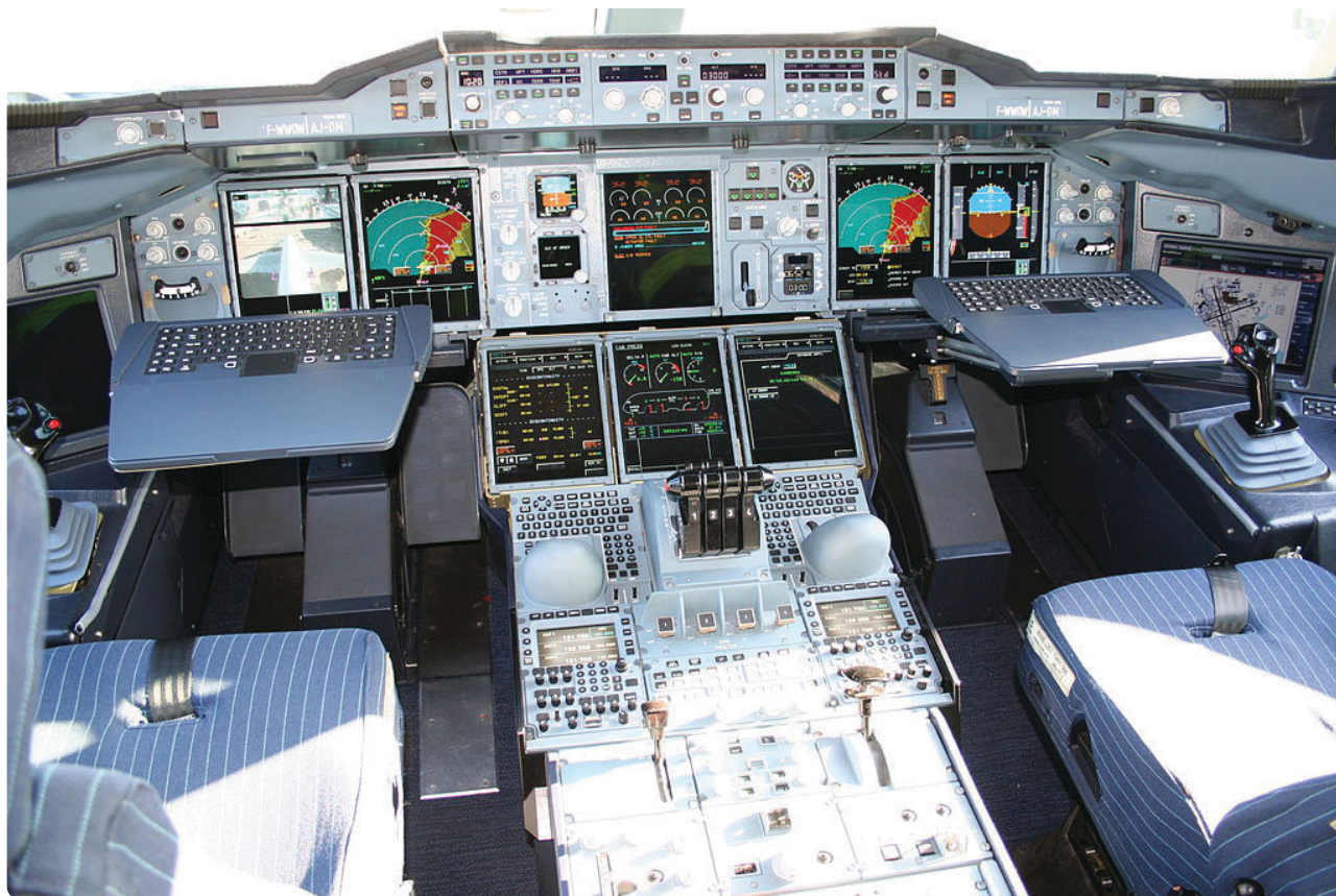
Figure 1-2. Airbus A380 EIS with 8 large LCD displays.
