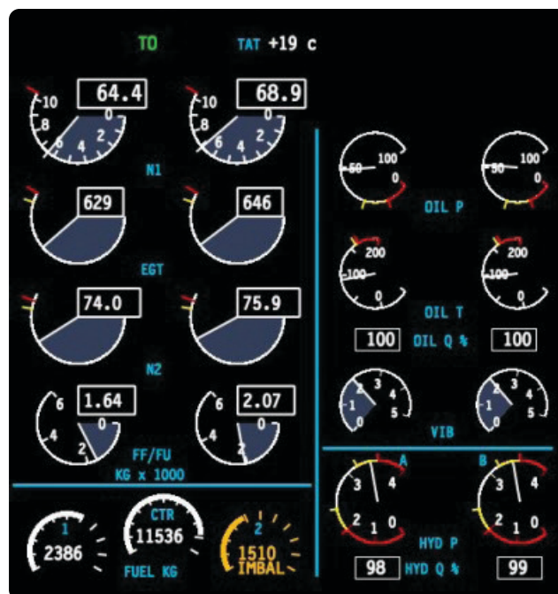
Figure 1-9. EICAS engine display format.
