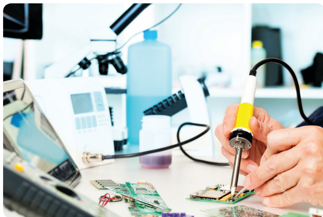
Figure 2-12. Repair of a printed circuit board.
