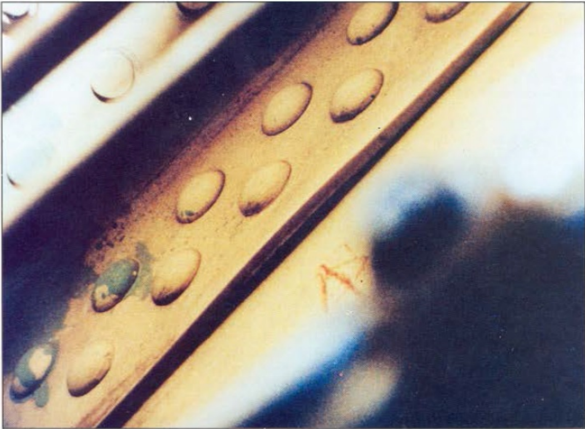
Figure 4-12. Skin Bulging Around Fasteners
