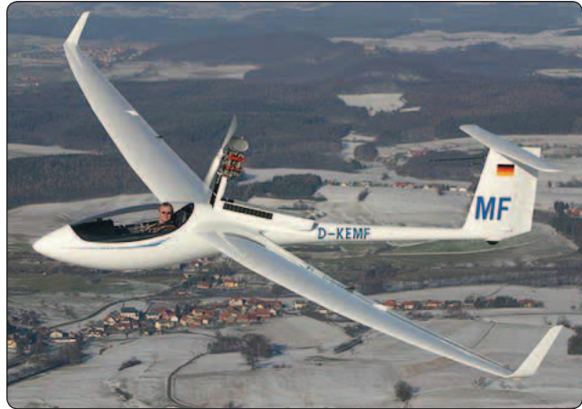
Figure 2-17. A Schleicher ASH 26e motor glider with the sustainer engine mast extended.
