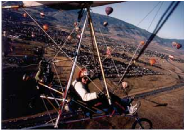
Figure 1-11. An ultralight vehicle trike: a Rogallo wing on a modified undercarriage.
