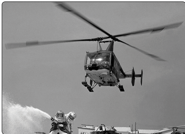
Figure 1-8. HH-43 Huskie with intermeshing rotors.
