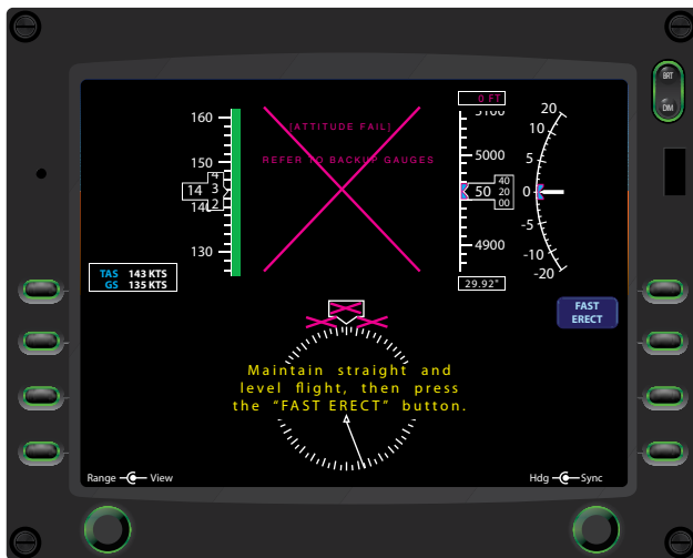
Figure 2-8. A PFD indicating a failed AHRS.
