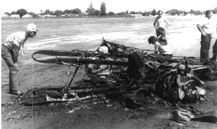
Pitts Special that crashed in a flat inverted spin following an entry from nearly zero airspeed. Film analysis shows that the pilot made three recovery mistakes: He applied and held full forward stick; he added full power, which caused the spin to go flat; and he attempted to use ailerons in the recovery.
