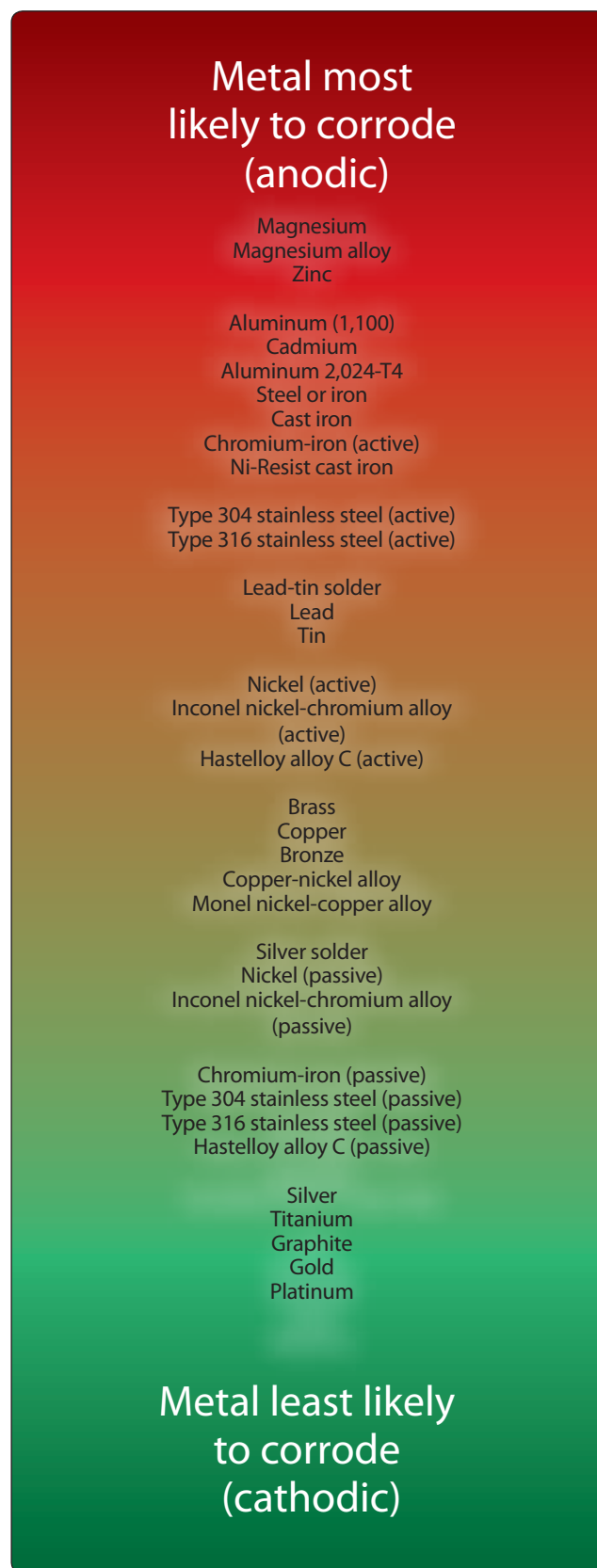
Figure 8-6. The galvanic series of metals and alloys.
