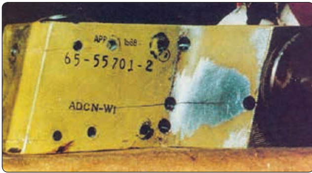
Figure 8-16. Stress corrosion cracking.
