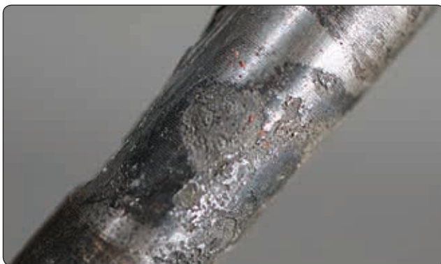
Figure 8-10. Dissimilar metal corrosion.
