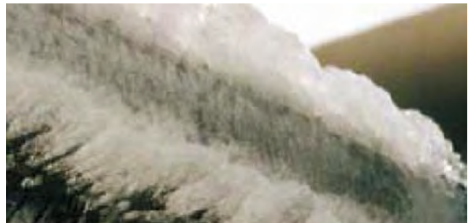
Figure 2-23. Inflight ice formation adds weight, increases drag and reduces lift.
