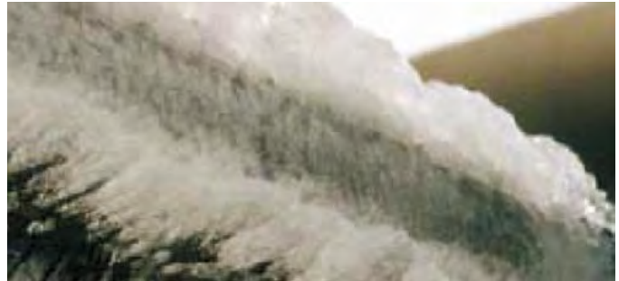
Figure 2-26. Inflight ice formation adds weight, increases drag and reduces lift.
