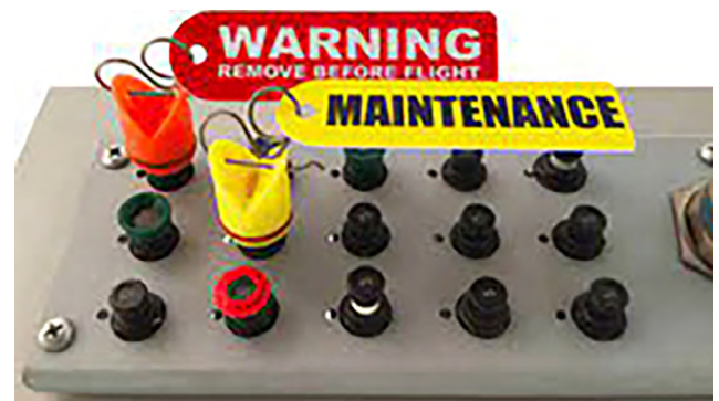
Figure 4-6. A circuit breaker panel with the critical system breaker locked and tagged.
