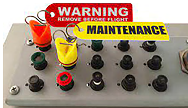
Figure 4-6. A circuit breaker panel with the critical system breaker locked and tagged.
