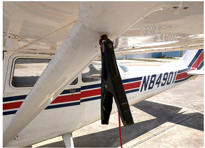
Figure 4-10. Grounding an aircraft (of any type) is a critical step during all fueling or defueling procedures.
