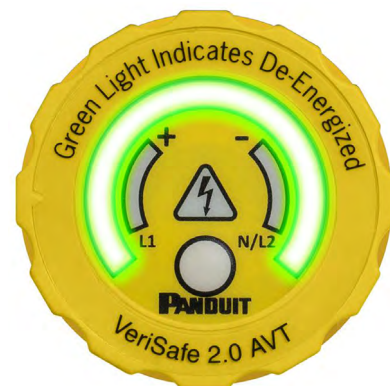
Figure 4-19. An Absence of Voltage Tester, if installed in the system or component is an acceptable and fast way to determine that the system is deenergized.
