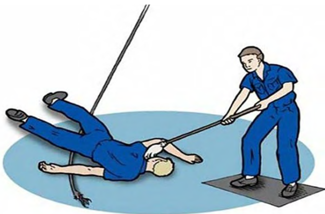
Figure 4-14. Never touch a person exposed to electricity. Use a non-conductive (wood) rod to separate them from the electrical source.
