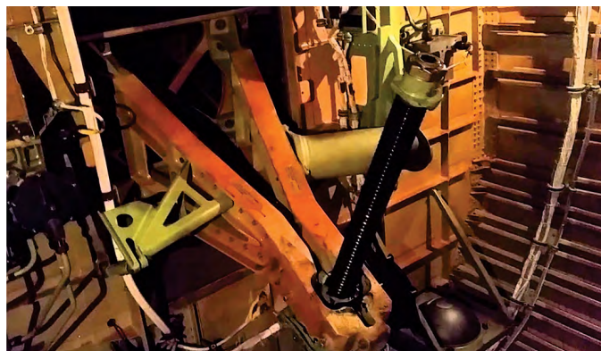
Figure 12-7. A jackscrew control arrangement on a Boeing 737-NG horizontal stabilizer.
