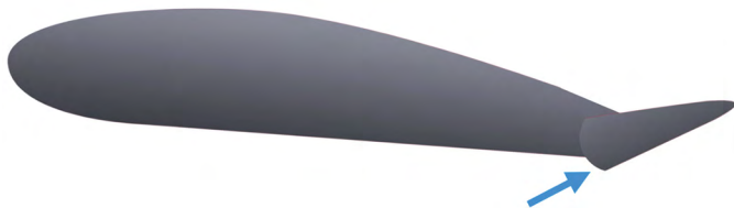
Figure 3-38. The bottom of the up aileron pivots into the airstream creating drag and helping to prevent flutter.
