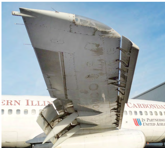
Figure 9-8. Outboard Trailing Edge Flaps and Slats Extended. Note how the extension of the flaps and slats increase the surface area of the wing in addition to altering the shape of the wing to enhance low-speed performance and lift production.
