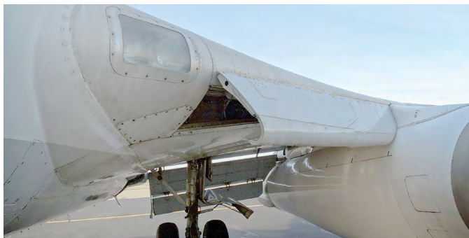
Figure 9-9. Leading edge and trailing edge inboard flaps extended. In addition to the outboard trailing edge flaps and slats shown in the previous illustration, leading edge flaps and inboard trailing edge flaps, seen behind the landing gear, are extended to further enhance low-speed performance.
