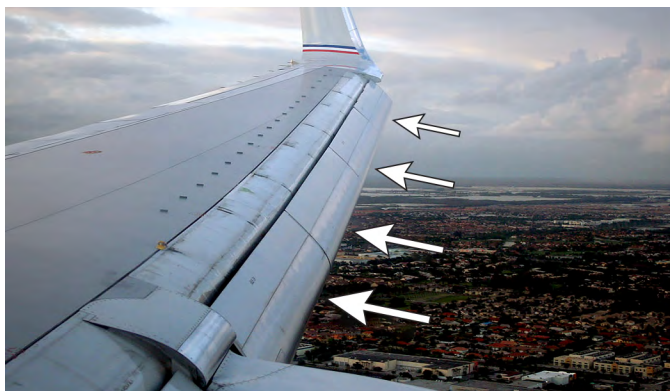
Figure 9-10. Leading edge slats deployed in low speed takeoff and landing position.
