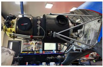
Figure 3-43. A turboprop engine mount with vibration isolation, in front of a stainless steel firewall.
