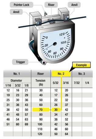
Figure 9-13. Cable Tensiometer and conversion chart.
