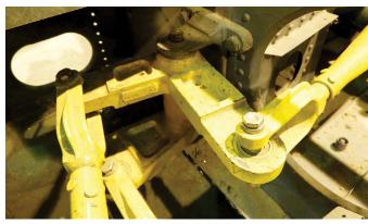
Figure 9-16. Bell crank with push-pull tubes.
