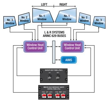
Figure 12-26. Electric window heat synoptic diagram for a Boeing 777.
