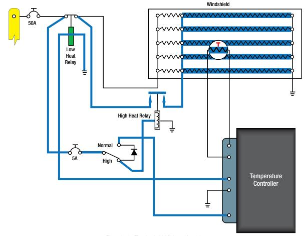
Figure 12-25. Electric windshield heat schematic.
