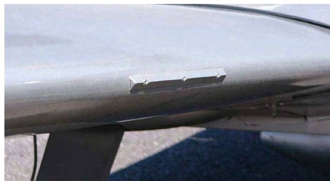
Figure 1-38. A stall wedge causes the wing root to stall before the outboard wing. This preserves airflow over the ailerons for controlled recovery from the stall.
