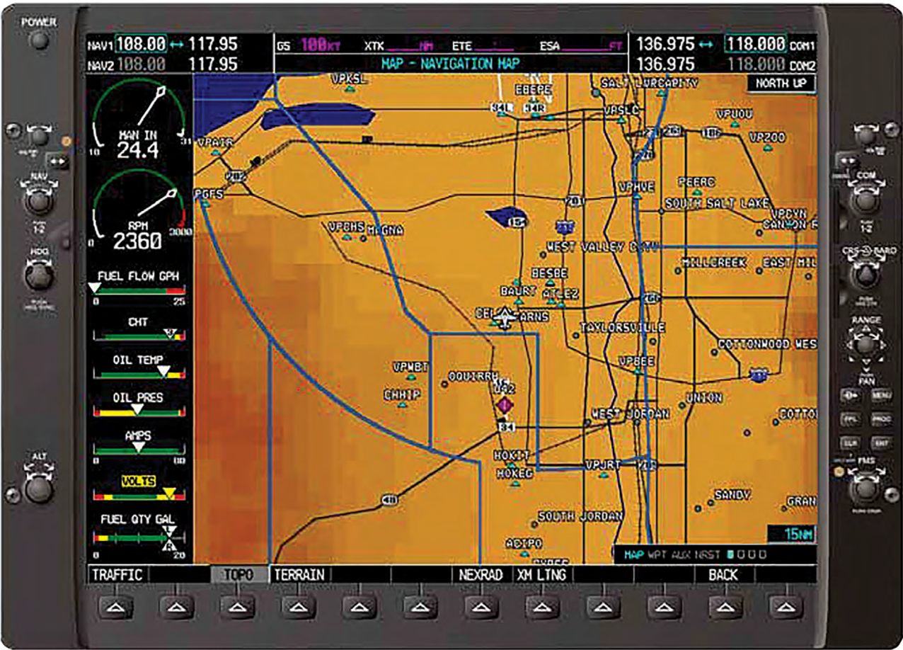
Figure 5-68. Oil pressure indication with other engine-related parameters shown in a column on the left side of this digital cockpit display panel.
