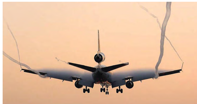
Figure 1-39. Vortices on an MD-11.
