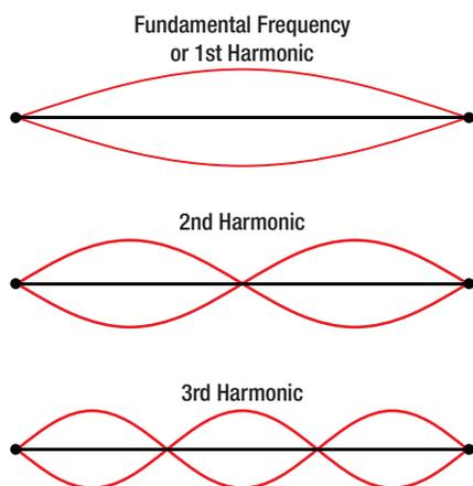
Figure 2-13. The first three levels of harmonic vibration.
