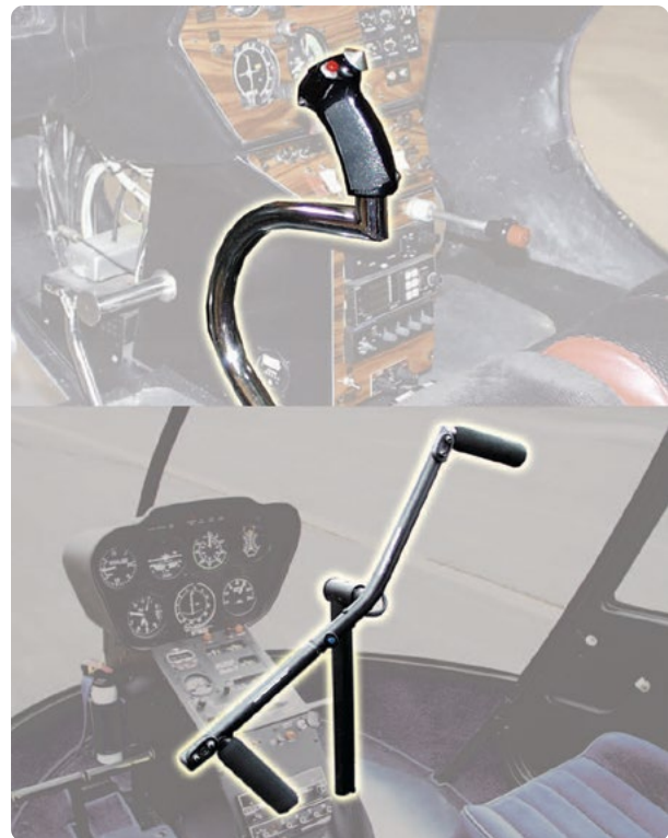
Figure 2-2. Location of cyclic pitch control.
