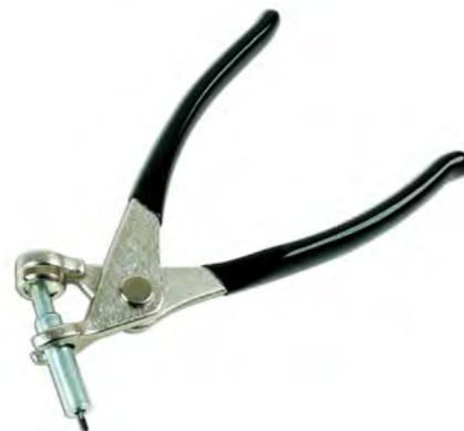
Figure 8-17. Celco pliers ready to insert a 3/32" cleco fastener.
