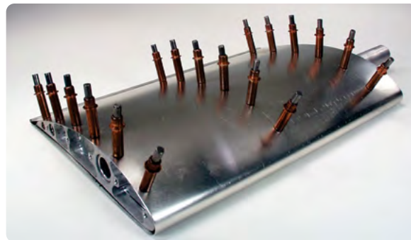
Figure 8-16. A part temporarily held together with Cleco fasteners.
